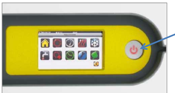
Figure 1: ON / OFF push-button switch (see pointing arrow) Switch lights => Power on (normal operation))
