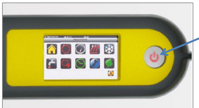
Figure 22: ON / OFF switch (see pointing arrow) Switch lights => Power on (normal operation)
